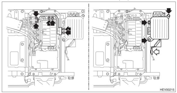
(5) Remove the inverter spacer from the electric oil pump inverter as necessary.
