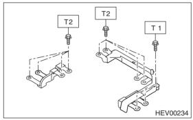
3) Install the inverter shield.
