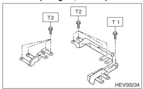
3) Install the inverter shield.
